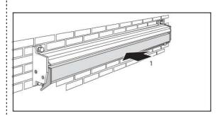
14. You may need to adjust the front plate to ensure a snug fit. (do not loosen completely)
