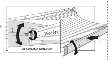
15. Once adjustments have been made it important to tighten the frontbar connection sufficiently.
