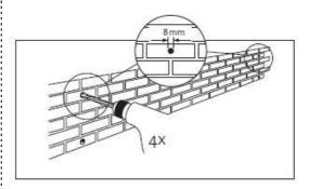
4. Screw the top two fixings into the wall leaving a gap of 3cm. 5. Lift the awning onto the fixings. 6. The awning should be fully closed. Ensure that the endplates are level. Insert the remaining two fixings and tighten all of them.
