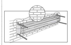
3. Drill an 8mm hole in the brick for each fixing point. The fixings provided will screw directly into the brickwork.
