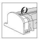
2. There should be at least 5 courses of bricks above the awning. If there is not then you should consider using spreader plates to bring the fixings further down the wall
