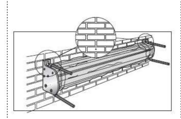
3. Drill an 8mm hole in the brick for each fixing point. The fixings provided will screw directly into the brickwork.
